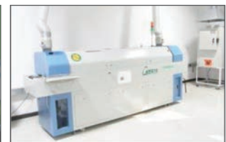
For SMD type products, simulating IR RELOW testing / 高溫無鉛回流焊機 (晉力達)
